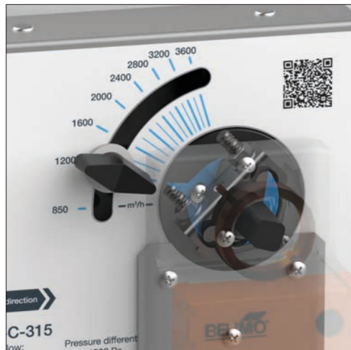
9. Unscrew the handle, press and hold the black button and set the indicator on the wanted minimal air flow value. In this case we will set it to the 1200 m 3 /h. Release the button and tighten the handle again
