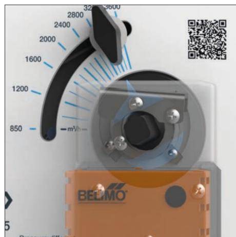
11. Unscrew the handle, press and hold the black button and set the indicator on the wanted maximum air flow value. In this case we will set it to the 2600 m<sup>3</sup>/h. Release the button and tighten the handle again
