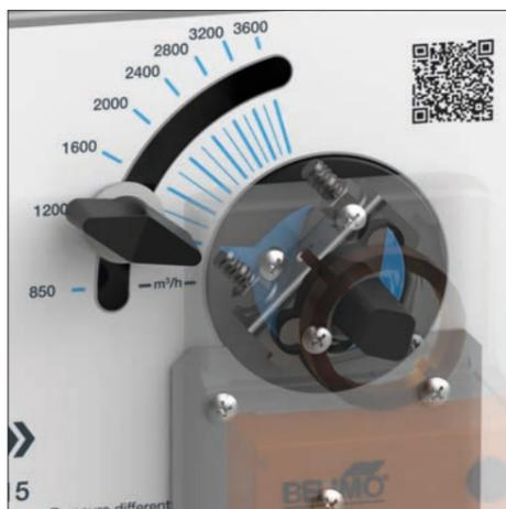
9. Unscrew the handle, press and hold the black button and set the indicator on the wanted minimal air flow value. In this case we will set it to the 1200 m<sup>3</sup>/h. Release the button and tighten the handle again
